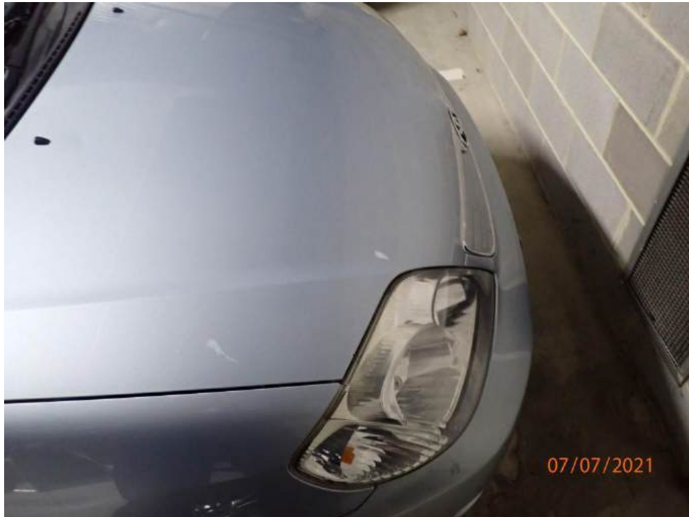
Photograph 7 - Calcium deposits on the bonnet of vehicle located at carpark 70
