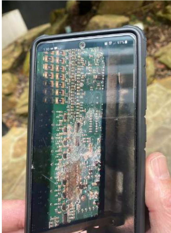
Corrosion to lift circuit board
